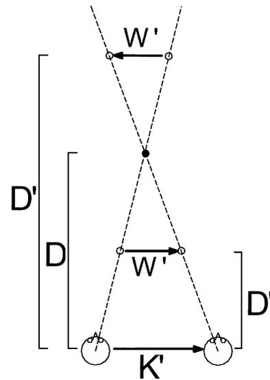
**Fig. 1** Apparent concomitant motion for a single point. When its distance is under-perceived ( $D'$ ), it appears to move in the same direction as head motion. When distance is over-perceived, it appears to move opposite head motion
